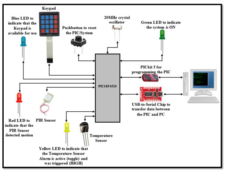
Note: \*The entire Alarm System circuit will be powered through the power provided by the USB-to-Serial Chip (FT232RL) coming from the computer's USB connection (no battery or direct wall power adapter is needed).
