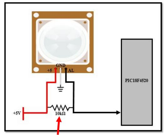
Note: Use an  $8.2k\Omega$  resistor instead of the  $10k\Omega$  shown here.
